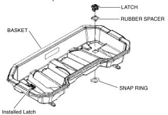
3. Lift the lever on each latch to unlock them. Place the utility basket onto the rear rack of the ATV. Line up each latch with its corresponding hole in the rack then push each latch into its hole.
