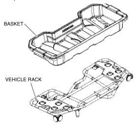
4. Secure the cargo box to the vehicle by pressing down each Honda Pro-Connect™ latch lever.
